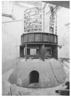
The hydroelectric plant featured new vertical turbines of the reaction type with a rated power of 4,500 horsepower each. Photo courtesy of the author.
